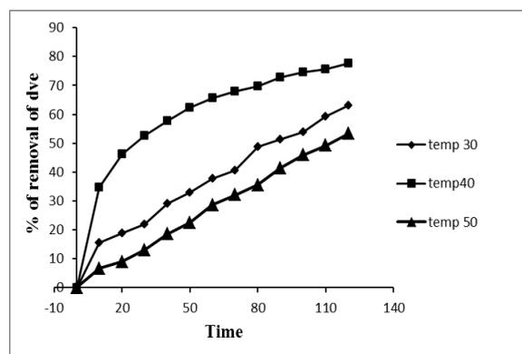
Figure - 5: Outcome of temperature on methylene blue adsorption on activated carbon.
