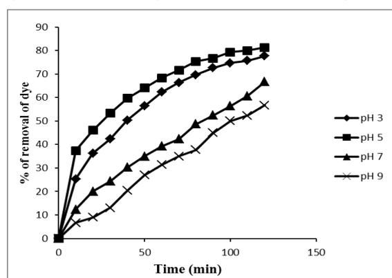
Figure - 3: Effect of pH on % of removal of dye by activated carbon.
