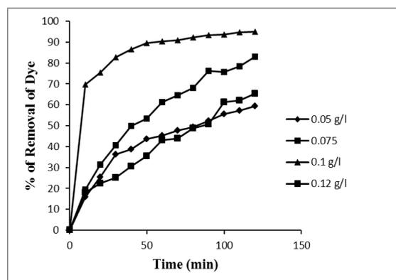
Figure - 2: Effect of various adsorbents (activated carbon) on % of removal of dye.
