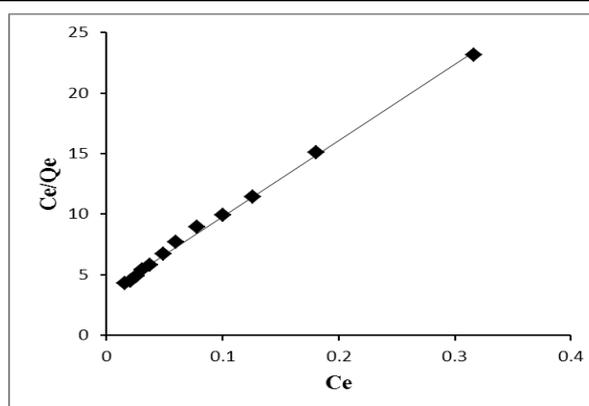
Figure - 7: Langmuir adsorption isotherm for adsorption of methylene blue on Activated carbon.
