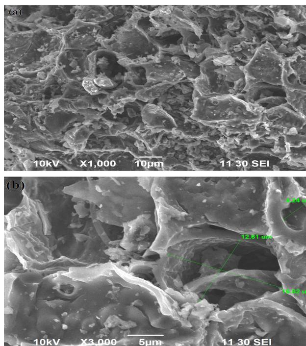
**Figure - 1: SEM image of activated carbon formed from *shorea roxburghii* (a) REPWM (b) activated carbon.**
