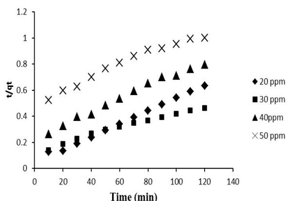
Figure - 9: Pseudo second order adsorption kinetics plots for the adsorption of methylene blue on activated carbon
