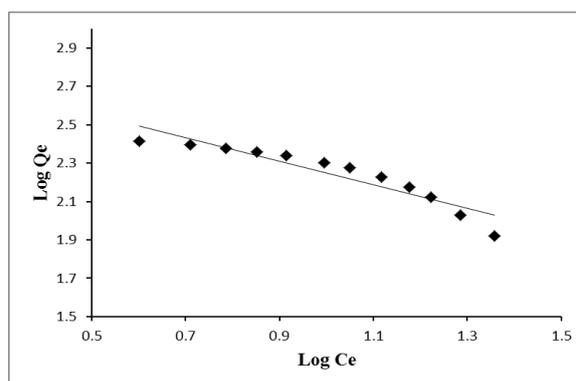
Figure - 6: Freundlich adsorption isotherm for adsorption of methylene blue on activated carbon
