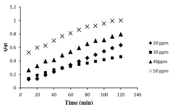
Figure - 8: Pseudo first order adsorption kinetic plots for the adsorption of methylene blue on activated carbon.
