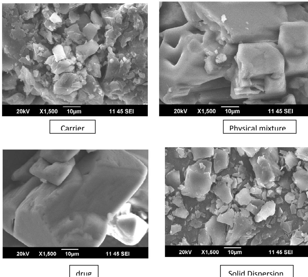
**Figure - 5: Scanning electron micrographs of carrier, physical mixture, pure drug and solid dispersion.**
