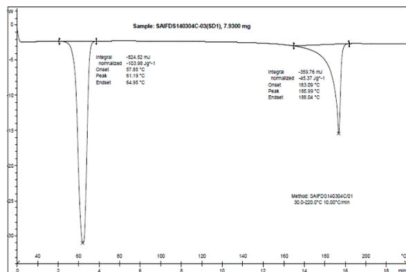
Figure - 2: The DSC thermograms of carrier(C1), satranidazole (S1), Physical mixture (PM1), and solid dispersion (SD1).
