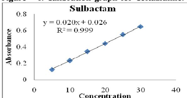
Figure - 5: Calibration graph for Sulbactam.
